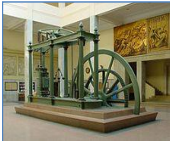
Figure 2.3b: A Watt steam engine. The steam engine, made of iron and fuelled primarily by coal, propelled the Industrial Revolution in Great Britain and the world.
